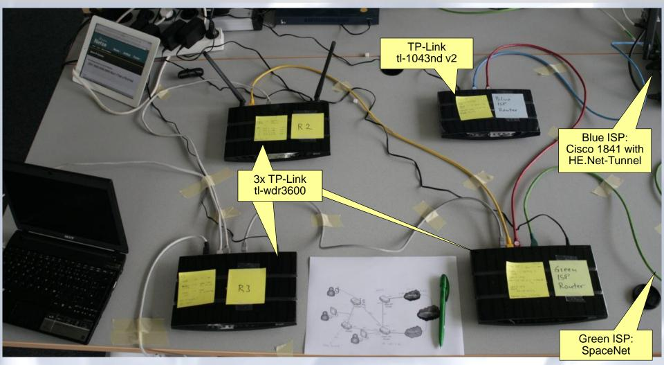
test platform: OpenWRT "barrier breaker" (trunk r40576), May 02, 2014
