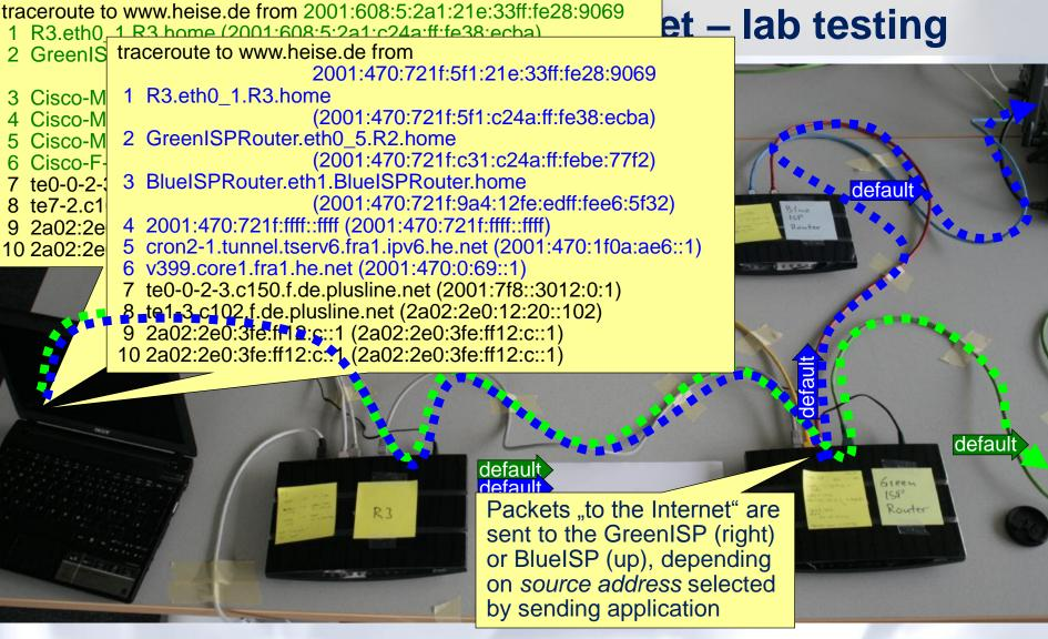
Routing in the Homenet based on target and source-address of packets
